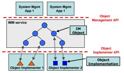
Figure 1: Schematic overview of the IMM.
